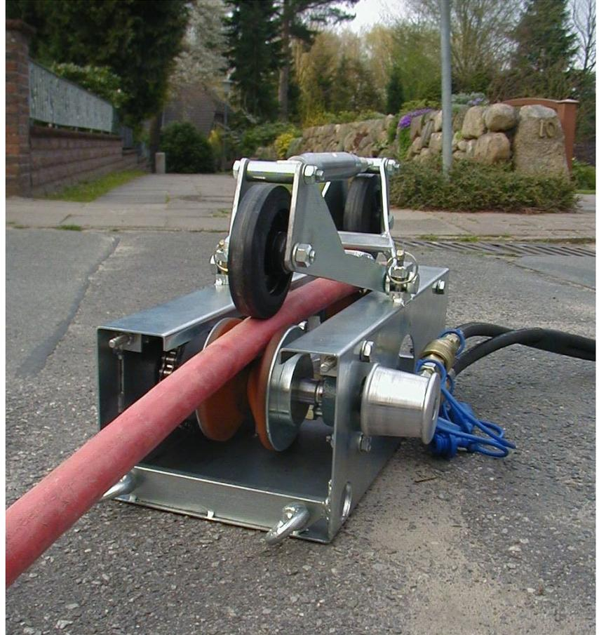
The Bagela cable and pipe pushing unit BKS 400 is designed for working sites with confined space, and is to be used also within buildings, power plants or on ships. It can be positioned directly into the cable tray because of the low weight and dimensions.
