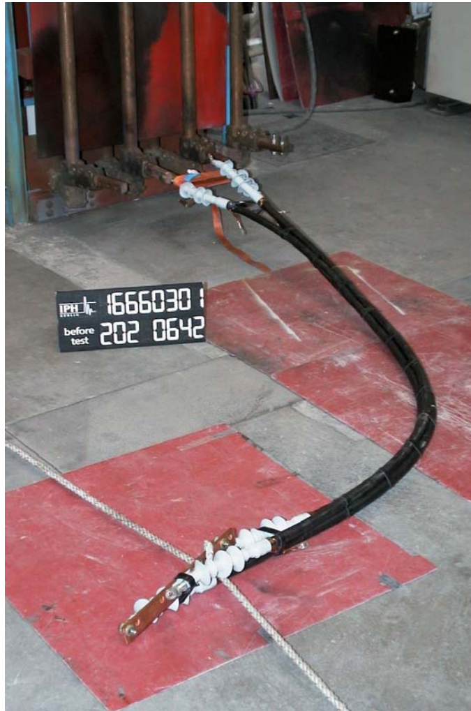
Figure 5: View of test objects before the dynamic short-circuit test
